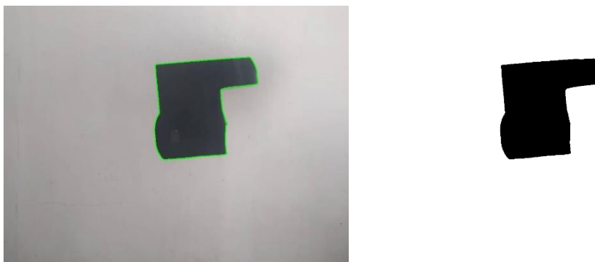
Fig. 8. White-black image (right) and edge detection (left) of the desired surface (second sample)
