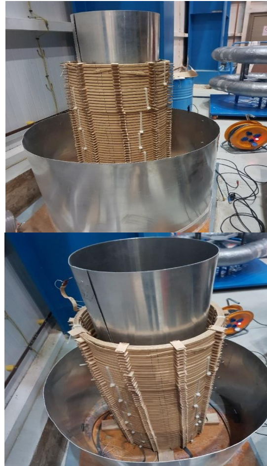
Fig. 6. 33 kV high voltage disc winding made specifically for this project.
