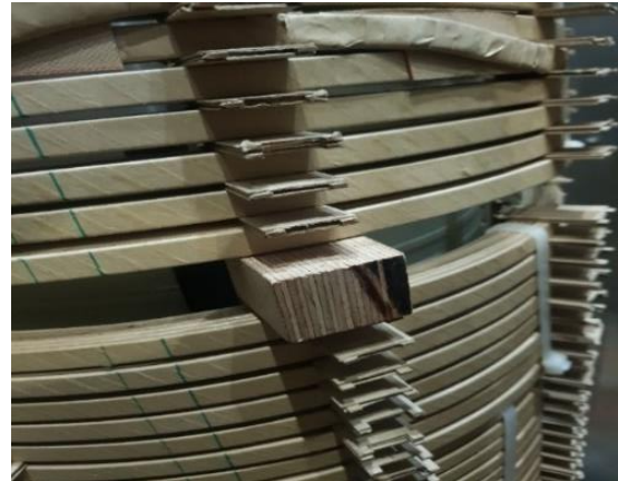
Fig. 7. Creation of axial displacement fault (axial deformation) on the studied winding.
