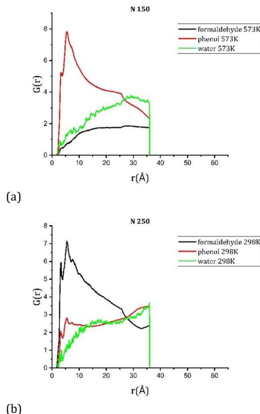
**Fig. 7.** Radial distribution functions for ternary mixtures of phenol, formaldehyde, and water adsorbed on the API 5L X70 steel surface: (a) 150 molecules of each component at 300 °C (573K) and (b) 250 molecules of each component at 25 °C (298K).
