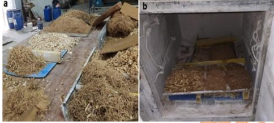
Fig. 1 (a) Fiber extraction, (b) heat treatment
