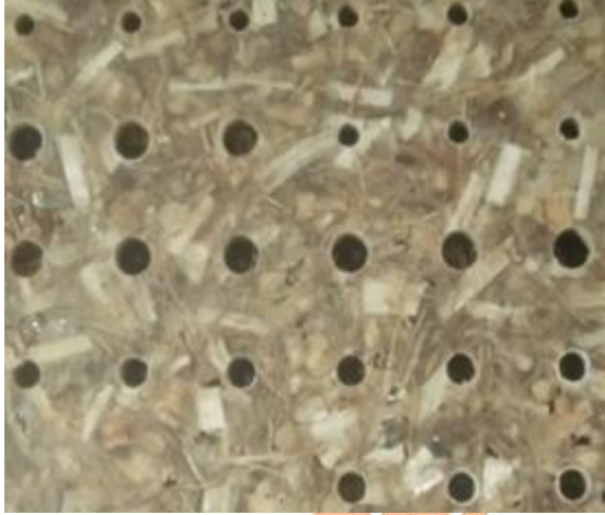
Fig. 4. Drilled laminate composite
