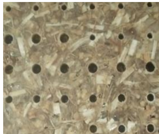
Fig. 4. Drilled laminate composite
