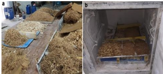
Fig. 1. (a) Fiber extraction, (b) heat treatment
