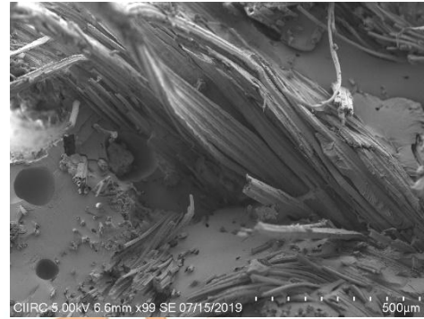
Fig.27 S5-10% Bamboo & 20% Jute Hybrid stacking sequence
