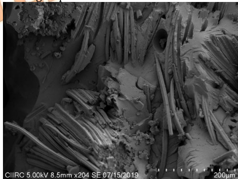
Fig.19 S4- 20% Bamboo & 10% Jute Hybrid stacking sequence
