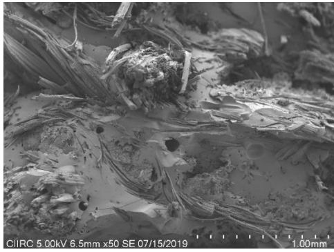
Fig.27 S5-10% Bamboo & 20% Jute Hybrid stacking sequence
