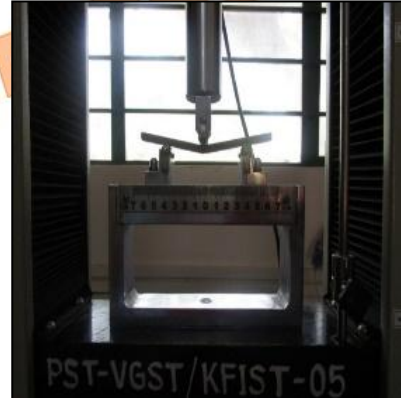
Fig 14. Computerized Flexural Testing Machine setup and specification of UTM
