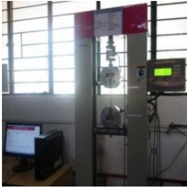
Fig 12. Computerised Universal Testing Machine for Tensile Test
