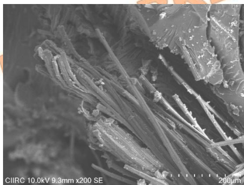
Fig.24 S1-10 % Glass, 10% Jute, and 10% Bamboo stacking sequence
