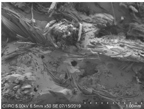
Fig. 26. S5-10% Bamboo & 20% Jute Hybrid stacking sequence
