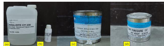
Fig. 3. Pictorial Representation of materials used in this study, (a) Epoxy Resin CY 230, HARDENER HY 951, (c) TOUGHENER I - CTBN, (d) TOUGHENER II - ETBN
