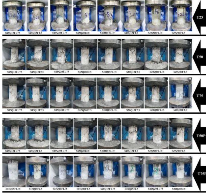
Figure 2: Crack and rupture pattern of experimental specimens
