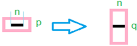
Fig. 2. Converting the RVE of SFRC to the RVE of a virtual long-fiber composite
