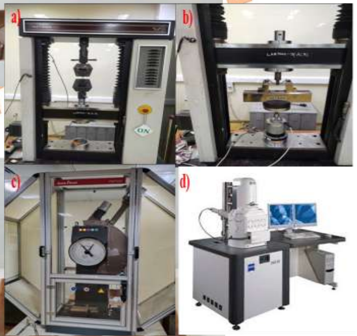
Fig. 5. Images of characterization apparatus (a) Tensile, (b) Flexural, and (c) Impact testing machine, (d) EDAX-SEM apparatus
