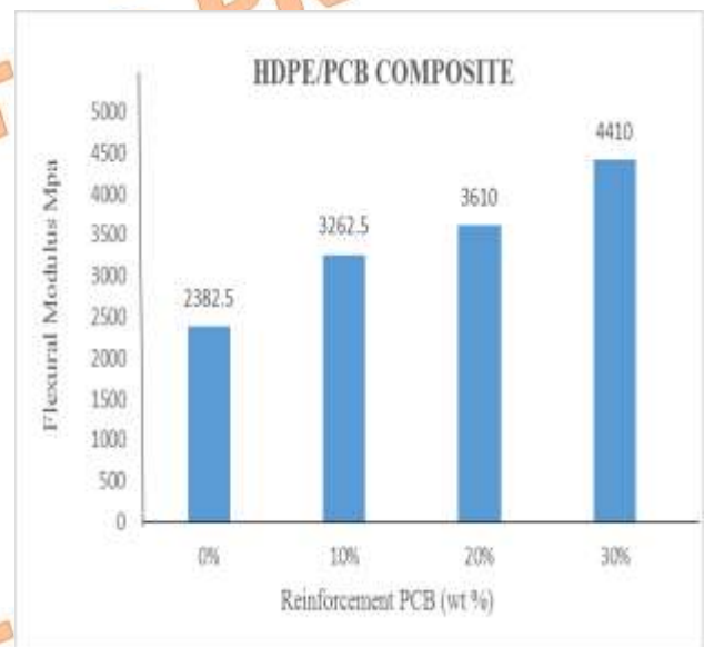
Fig. 12. Effect of reinforcement wt. (%) on Flexural strength
