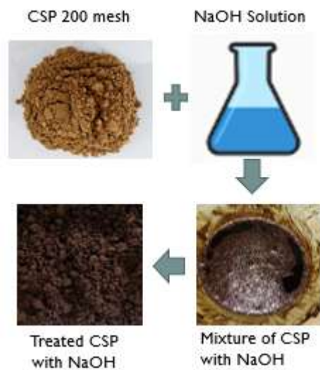
Fig. 2. Alkali treatment process of coconut shell particles through immersion in NaOH solution
