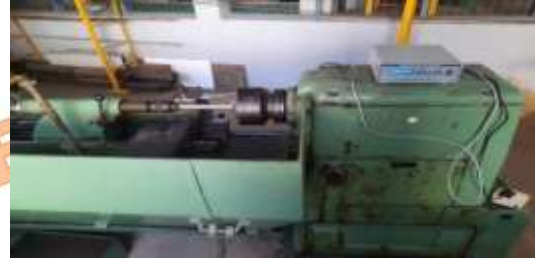
Fig.2. Semi-automatic lathe equipped with a lathe tool dynamometer
