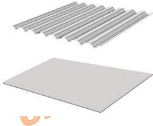
Fig. 3. Homogenization of corrugated sheet to equivalent orthotropic plate
