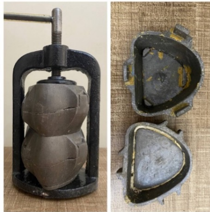
Figure 2: Plaster mold and metal cast used to cure PMMA
