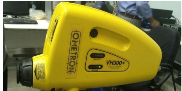
Figure 2: Vibration measured by the OMETRON VH300+ laser doppler vibrometer.
