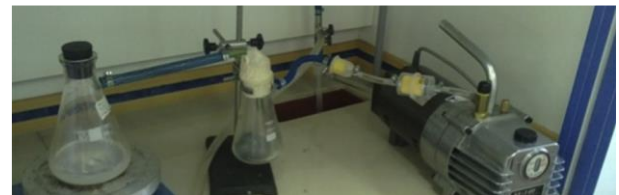
Figure 1: Mixing and solvent evaporation procedure under vacuum situation.
