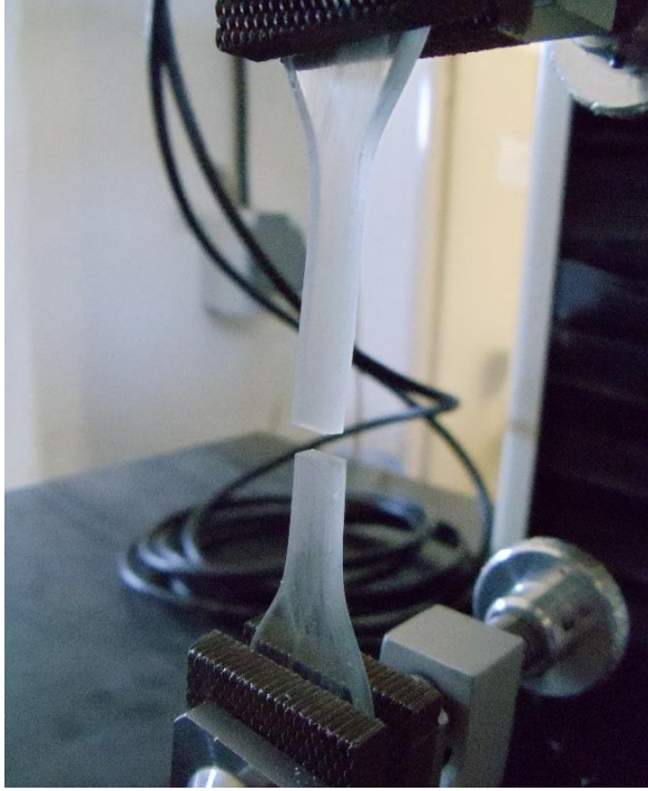
Figure 2. Picture of a pure resin sample after tensile testing
