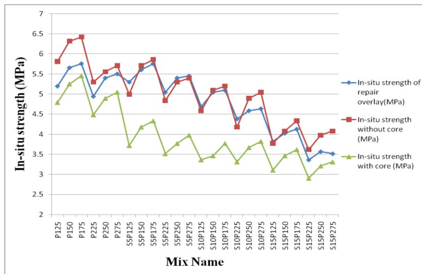
Fig.8 The comparison of three types of in-situ strength tests
