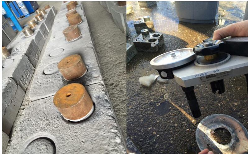
Fig. 1 Partial core drilled samples and the equipment for In-situ and Pull-off test
