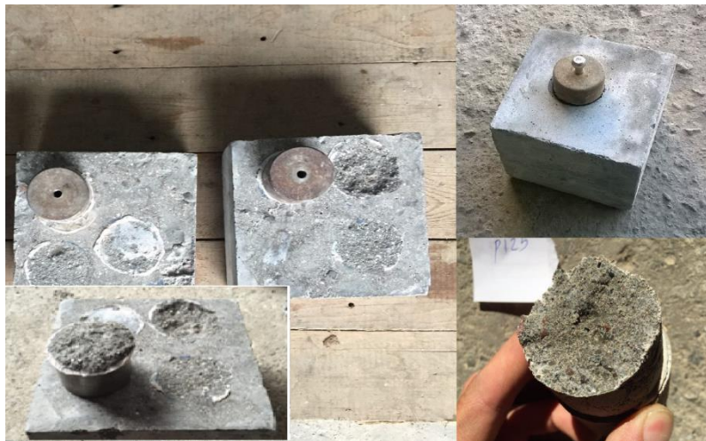
Fig. 2 In-situ test with core and without core drilling
