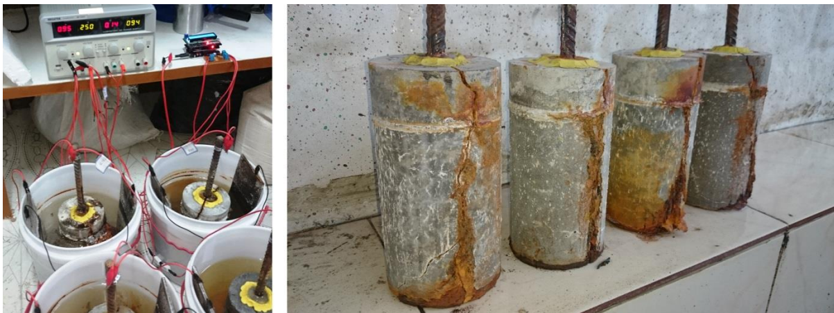
Fig. 10. Accelerated corrosion setup and typical corrosion specimens after the accelerated corrosion test
