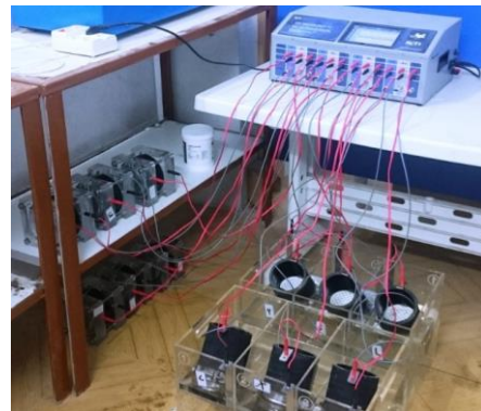
Fig. 1. Test setup of RCPT and RCMT
