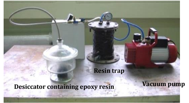
Figure 3. Degassing of the epoxy resin using a vacuum pump
