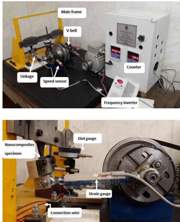
Figure 4. The experimental setup for the displacement controlled flexural bending fatigue loading
