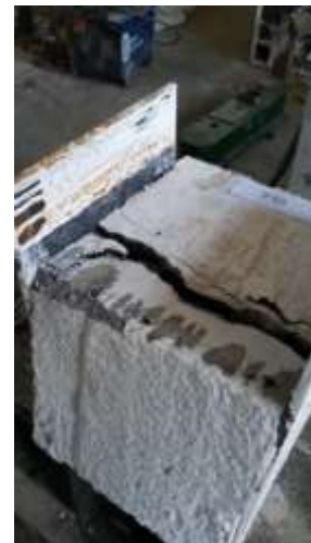
c. status of sample after failure
