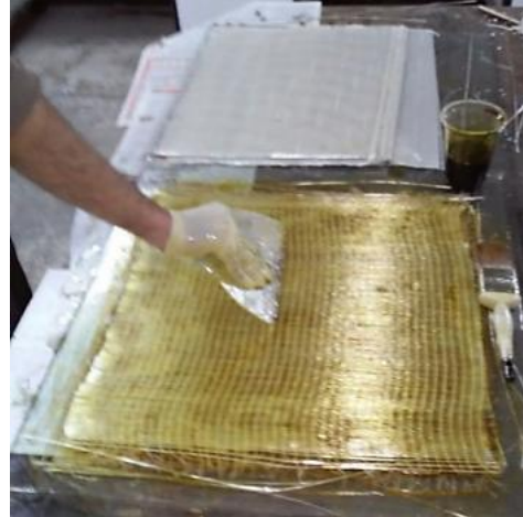
Figure 4. Epoxy impregnated UD e-glass fiber
