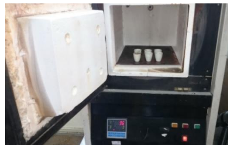
Figure 6. Putting the GFRP specimens in the furnace
