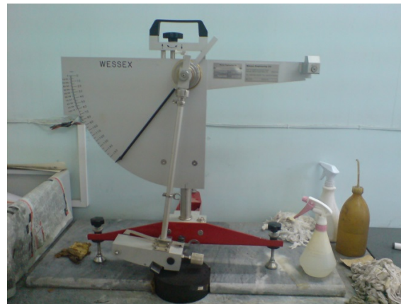
Fig. 3. Manner of Drawing up the Slip Length ( 125 \pm 1.6 Millimeter) on the British Pendulum Tester, with 15 cm Diameter Samples
