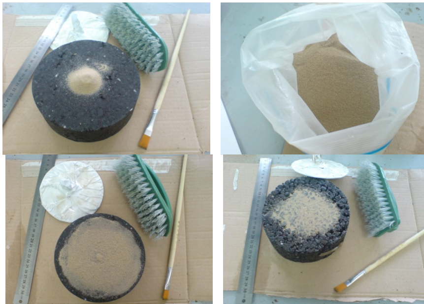
Fig 8. Preparation of river roundness sand passed through sieve No. 60 and retained on sieve No. 80 and distribution of specific volume of sand on the surface of the asphalt mix sample with open and dense grade
