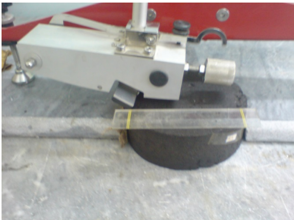
Fig. 3. Manner of Drawing up the Slip Length ( 125 \pm 1.6 Millimeter) on the British Pendulum Tester, with 15 cm Diameter Samples
