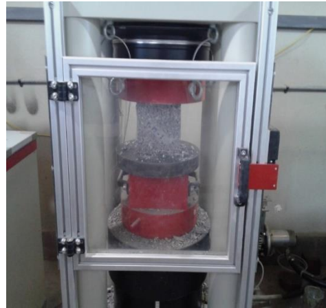
Figure 4. Load jack used to measure compressive strength
