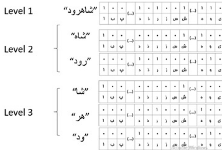
Figure 3: PHOC representation of SHAHROOD in three levels by Persian character set. All of partial histograms in all levels are concatenated to make final PHOC histogram.
