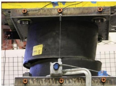
Fig. 5. Slip through failure mode in a post-cavitation lateral displacement test (axial pressure = 0.5 MPa), [27].
