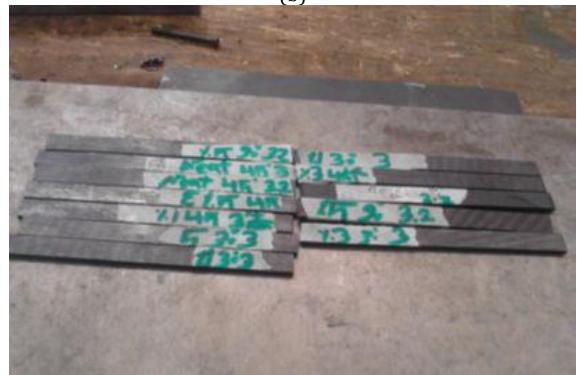
Figure 2. (a) the vacuum procedure and (b) the prepared samples after cutting with diamond blade saw.
