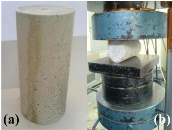
Fig. 3. (a) Cylindrical specimen and (b) Concrete Tensile strength testing machine.
