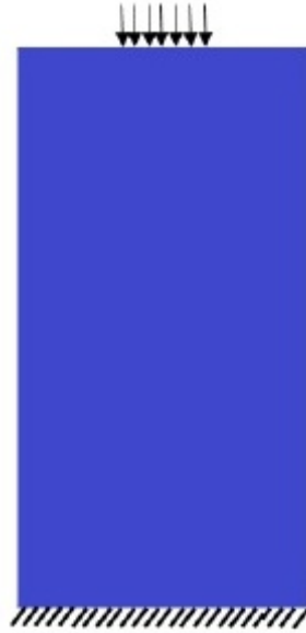
Fig. 3. One fixed end continuum structure under distributed load
