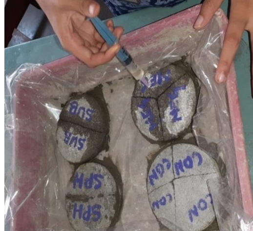
Fig. 8. Represents the mortar discs being injected with a bacterial solution.
