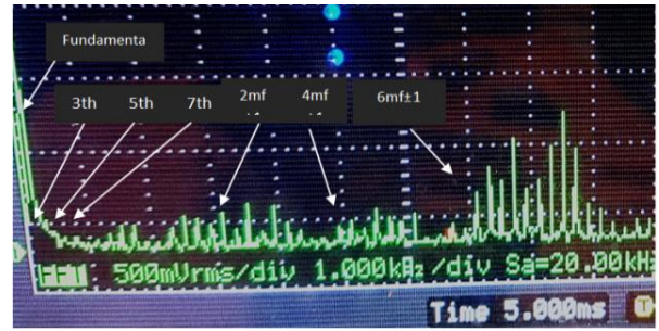
Fig (23): Harmonic analysis of the output waveform of the inverter on oscilloscope
