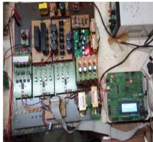
Fig (14): Fabrication of full bridge H cell on PCB.
