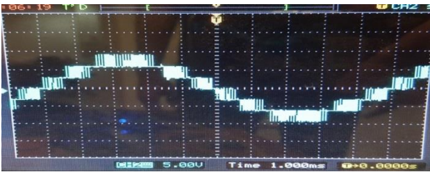
Fig (19): output waveform of the inverter with SPWM modulation- 1 cycle
