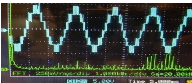
Fig (22): output voltage waveform of the inverter along with harmonic analysis
