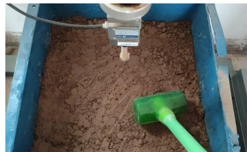
Fig. 11. Compaction of the clay layer.
