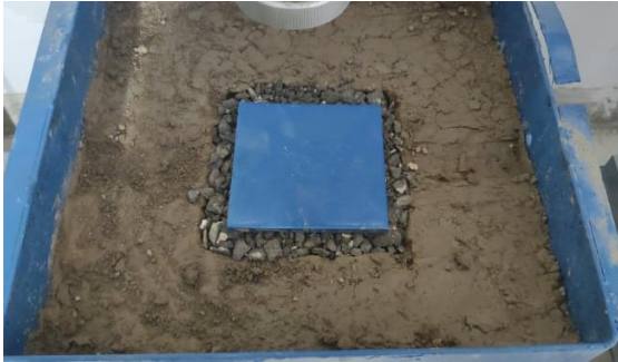
Fig. 13. RAP layer under the square footing.
