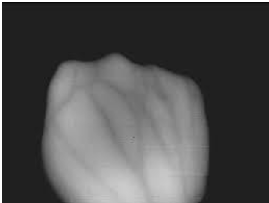
Figure 2: Hand vein using a monochrome NIR CCD camera
