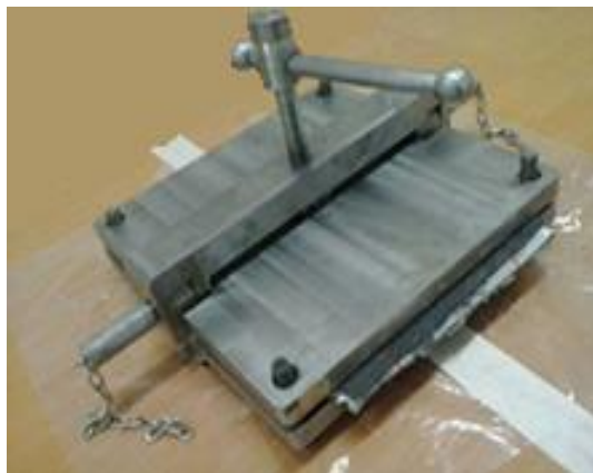
Fig. 4. Fabricated CFRP pressed in a fixture
