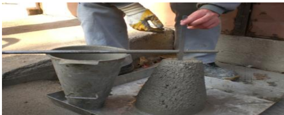
Fig. 3. Measuring the concrete slump
