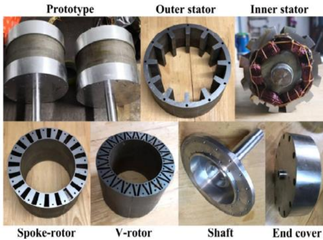
Fig.6. Various parts of DS-PMV machine [44]
