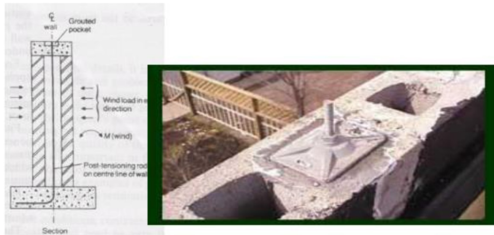
(a) Prestressed masonry diaphragm walls
