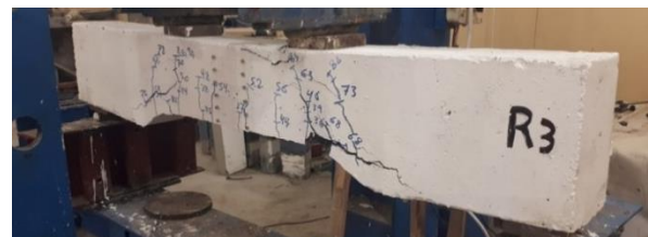
Fig. 9. Cracks pattern at failure for beam (R3).
