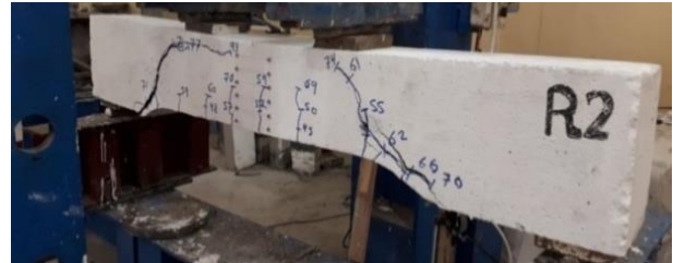
Fig. 8. Cracks pattern at failure for beam (R2).
