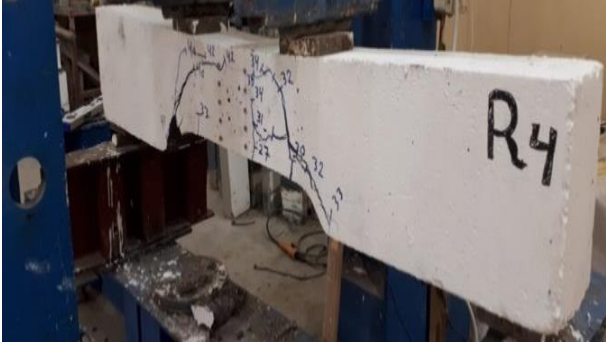
Fig. 10. Cracks pattern at failure for beam (R4).
