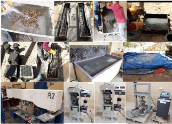
Fig. 6. Casting and curing process of beams.
