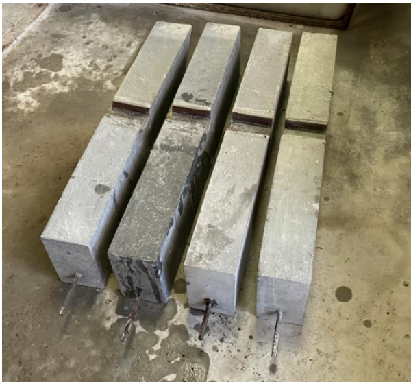
Fig 2. Prepared HPFRCC beam for beam-bending test.
