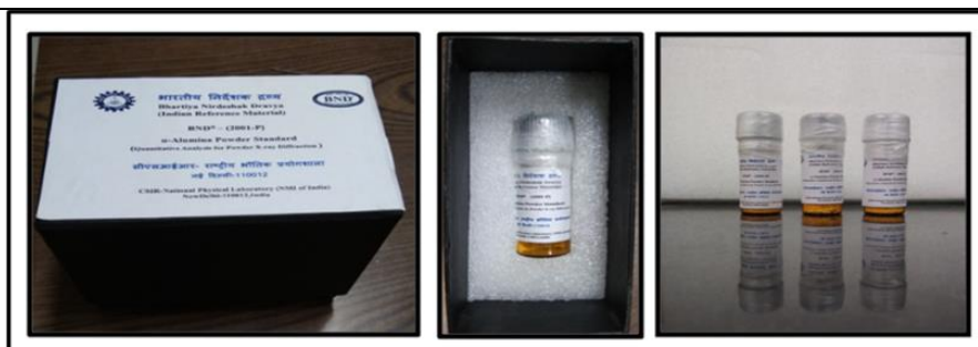
Fig. 10. α-Alumina: The Indian Reference Material for the calibration of PXRD.
