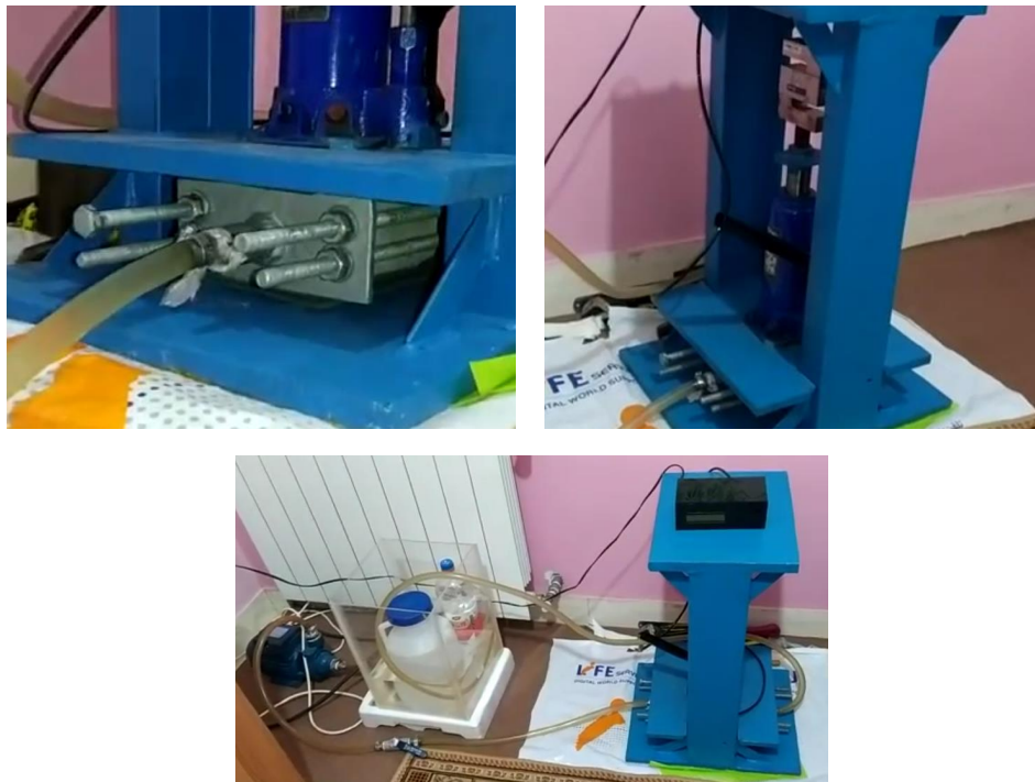
Figure 3: Apparatus for applying vertical overhead and circulation
