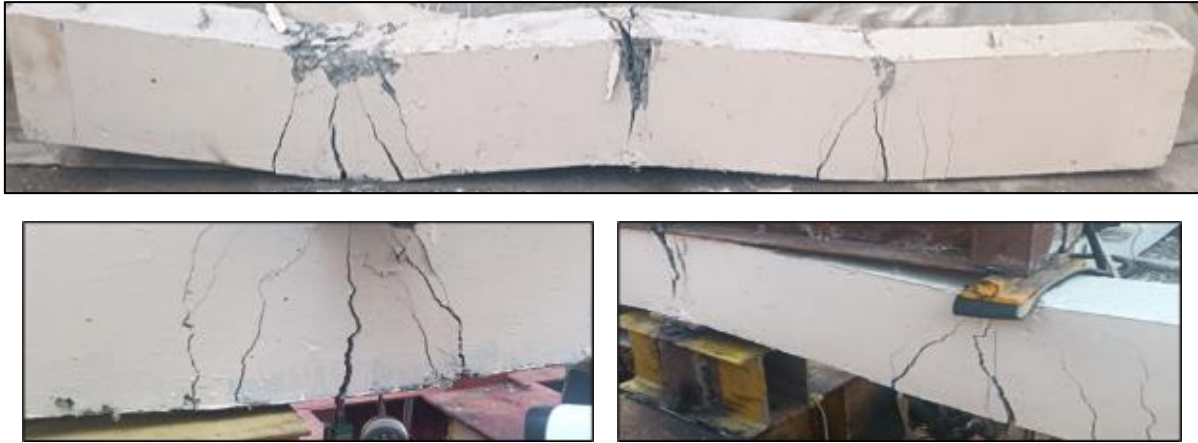
Fig. 10. Flexural Failure Mode, (CB).
