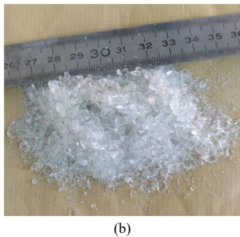
Fig. 1. Granular materials evaluated in this study: a- River sand category, b- Crushed waste glass.
