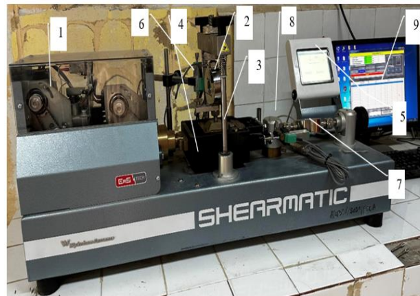
Fig. 5. Direct shear apparatus and the acquisition system used in the study.
