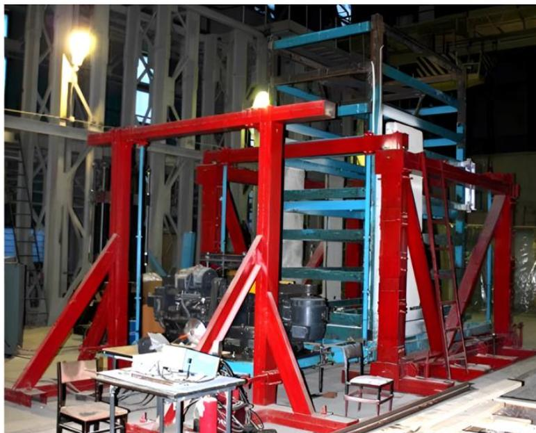
**Fig. 8.** Experimental equipment for assessing seismic resistance of developed hinged façade system [25].
