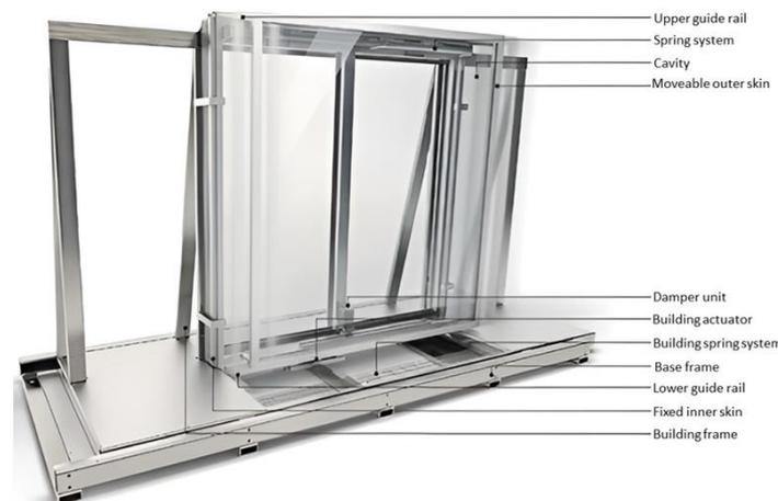
**Fig. 9.** The new semi-active distributed-multiple tuned façade damper [44].
