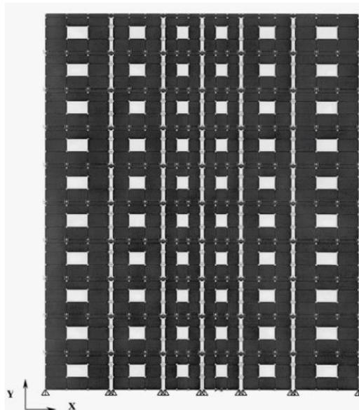
**Fig. 6.** 10 story precast concrete load-bearing panel facade using V joint configuration [24].
