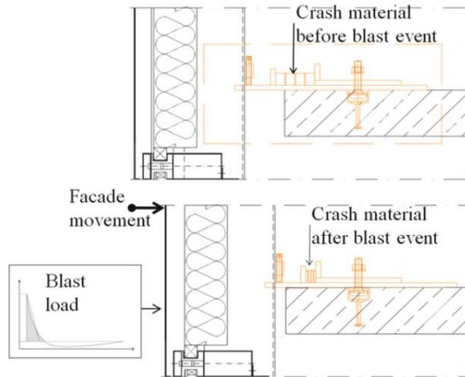
**Fig. 7.** Principle of dissipative façade brackets [41].
