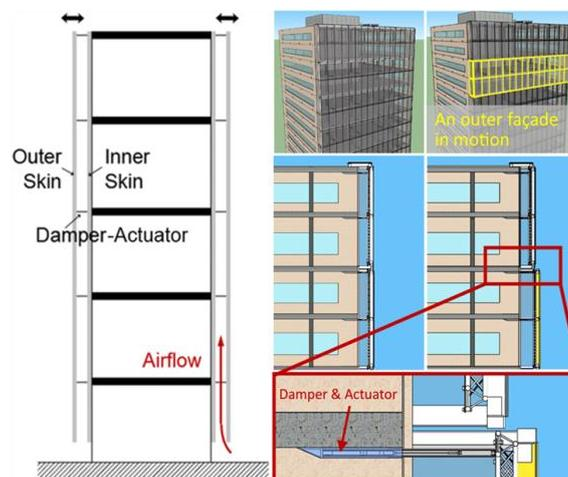
**Fig. 14.** Double-skin façades- damper system, motion of the double-skin façades system [43].
