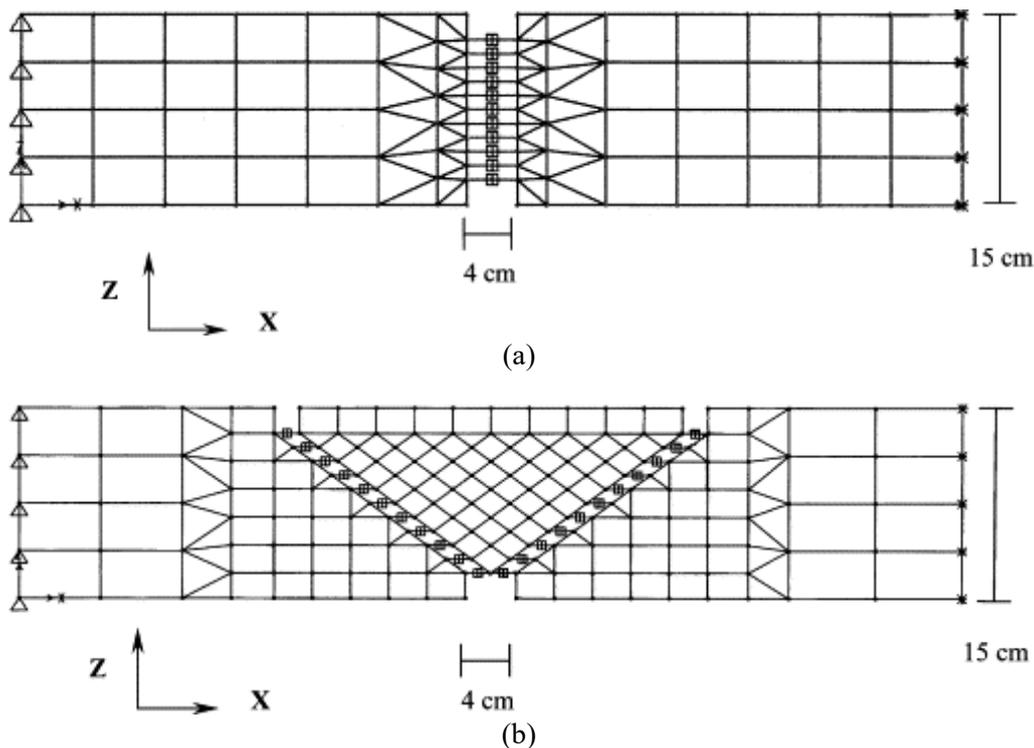
**Fig. 4.** (a) Finite element model of the flat-joint case; (b) Finite element model of the V-joint case as developed by Barluenga and Hernández-Olivares [24].
