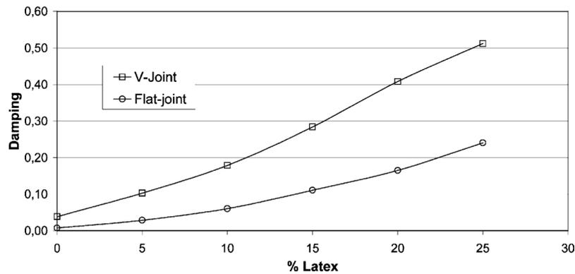
**Fig. 3.** Damping energy of flat joint and V joint for various percentages of latex-modified mortar [24].
