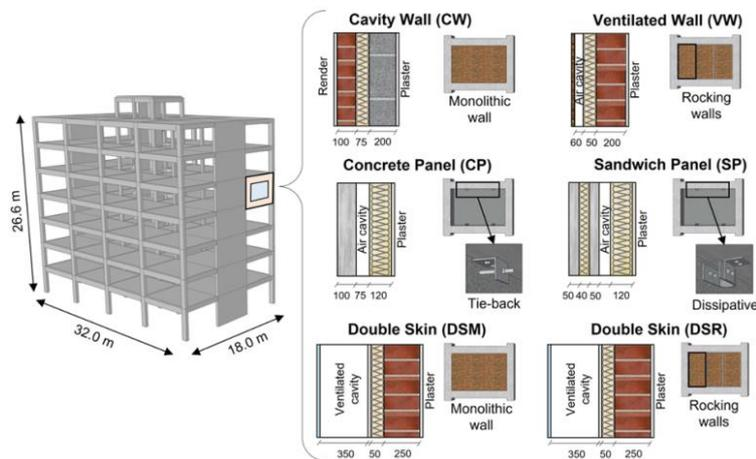
**Fig. 11.** Alternative façade design approaches [45].
