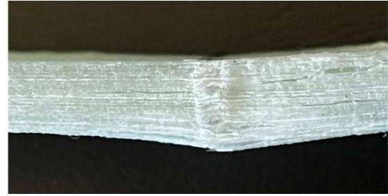
Fig. 3. Delamination of glass fiber laminate after 3-3PBT
