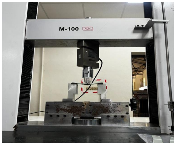
Fig. 2. Specimen mounted in UTM.
