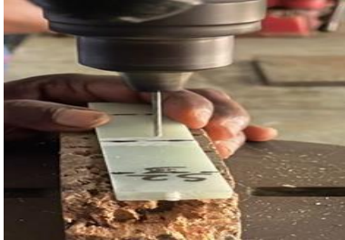
Fig. 1. Specimen drilled for Repair work.
