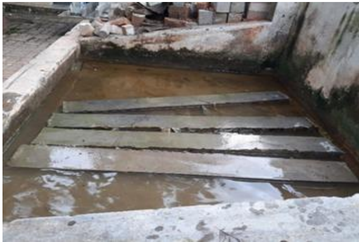
c) Curing of RC beams in a water bath.
