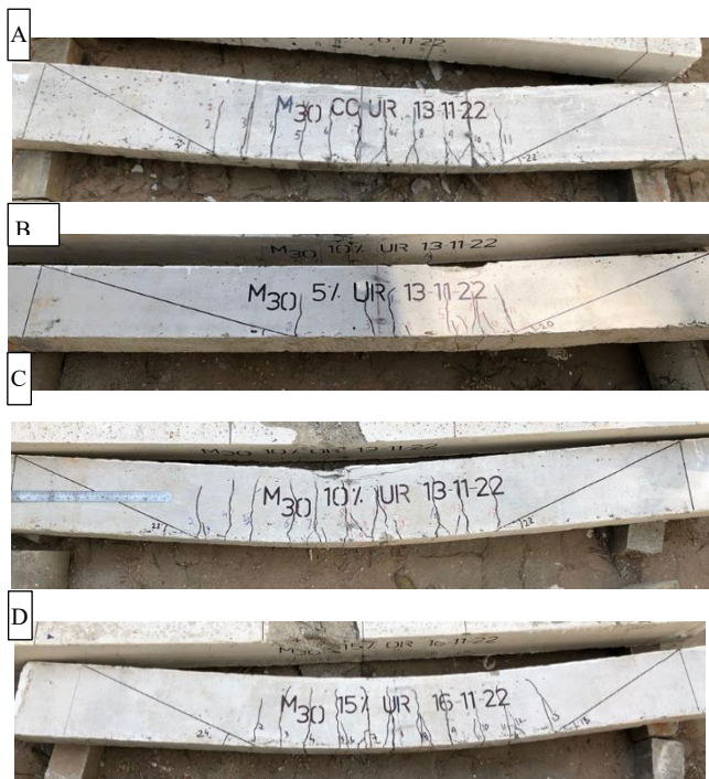
Fig. 6. The crack pattern of Alccofine-based M30 grade RCC beams for Under-reinforced case.
