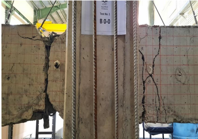
Fig. 5. Specimen No. 1 at the end of cycle 9, with a displacement of 70 mm (drift of 3.5%).
