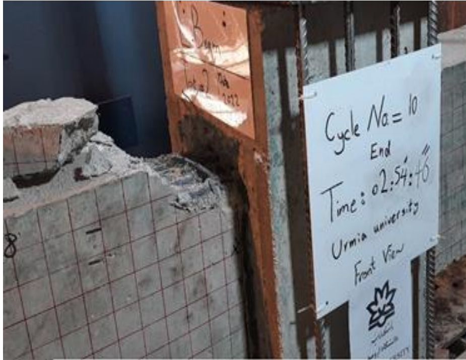
Fig. 10. State of the specimen No. 2 at the end of the test.
