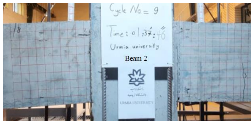
Fig. 8. State of specimen No. 2 at the end of load cycle 9 with a displacement of 70 mm (drift of 3.5%).
