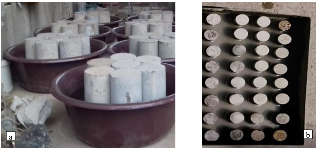
Fig. 2. Cylinders: (a) (100x200mm); (b) (38mm x 50mm) partially submerged in the curing mixture.
