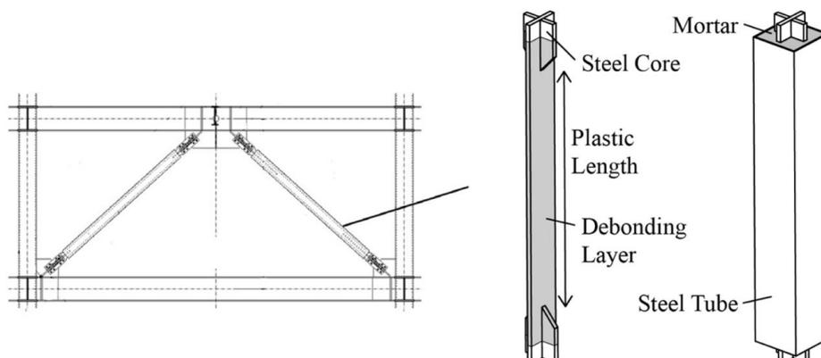
**Fig. 4.** Concept of buckling-restrained brace [30].
