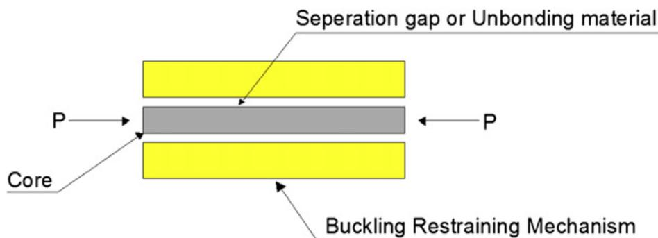
Fig. 2. Typical BRB member components [4].
