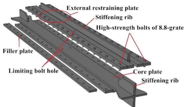
**Fig. 5.** Diagram of the all-steel assembled LYBR [51].
