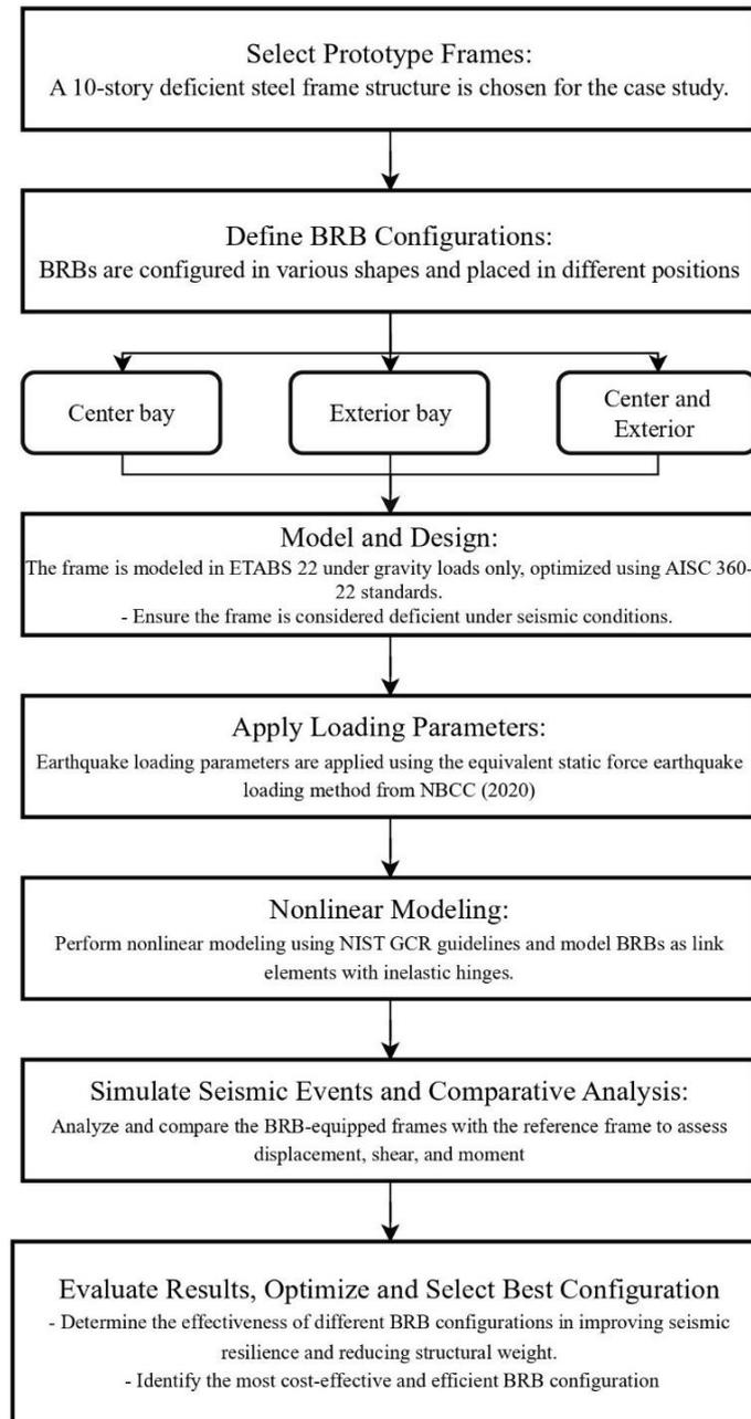
**Fig. 7.** Methodology and Process for Seismic Analysis of a 10-Story Deficient Steel Frame Structure with Buckling-Restrained Braces (BRBs).
