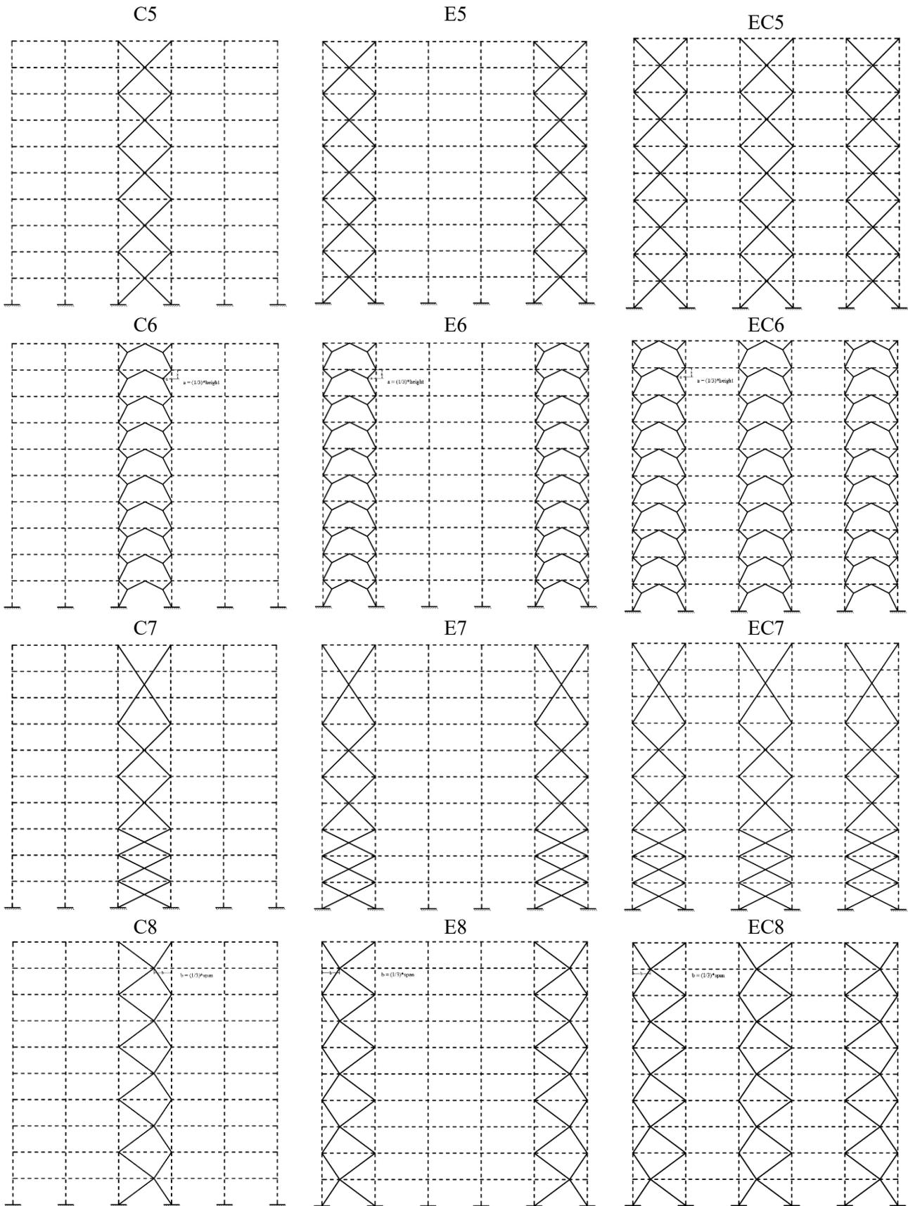
Fig. 7. Configuration of different studied frames equipped with buckling restrained braces.
