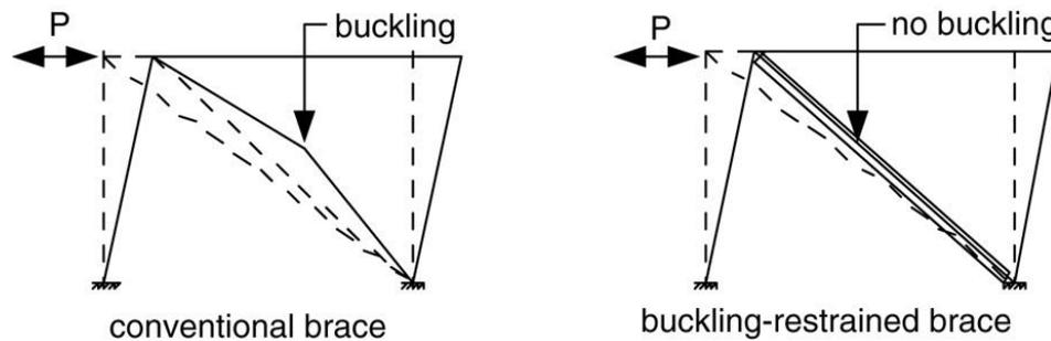
Fig. 1. Buckling behavior of conventional brace and BRB [3].
